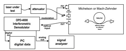
Laser under test is input to interferometer, which is set to the appropriate optical path mismatch by selection of the delay line which may be user installed or changed. OPD-4000 modulation output is applied to PZ1 fiber the OPD-4000 stretcher input. phase measurement output is selected as either digital or Digital data is post analog. processed. Analog data is made available to signal analyzer.
